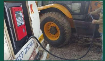
RFID enabled nozzle dispensing fuel from Bowser to equipment after reading RFID tag fitted in eqpt. fuel tank
